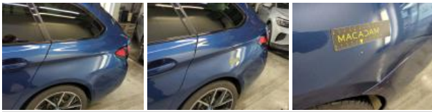
Door RL, Scratch(es), Repair and paint (complete)
