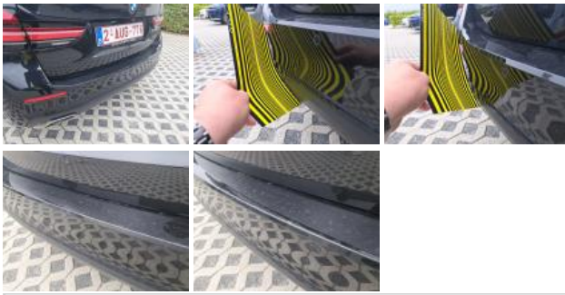
Wing RR, Dent(s), Paintless dent repair
