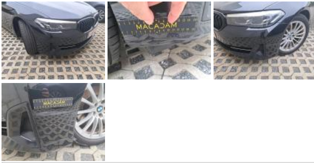
Bumper moulding F, Broken, Replace
