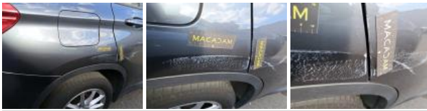
Door RR, Scratch(es), Repair and paint (complete)
