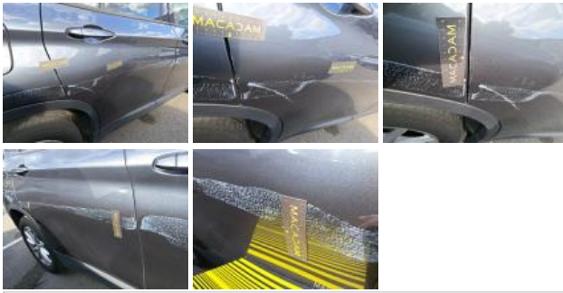
Door FR, Scratch(es), Repair and paint (complete)
