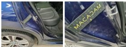
Roof pillar R, Chemical polution, Repair and paint (complete)
