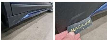
Door RR, Repaired, Acceptable
