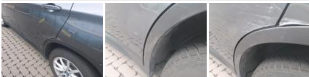
Door trim RL, Scratch(es), Acceptable
