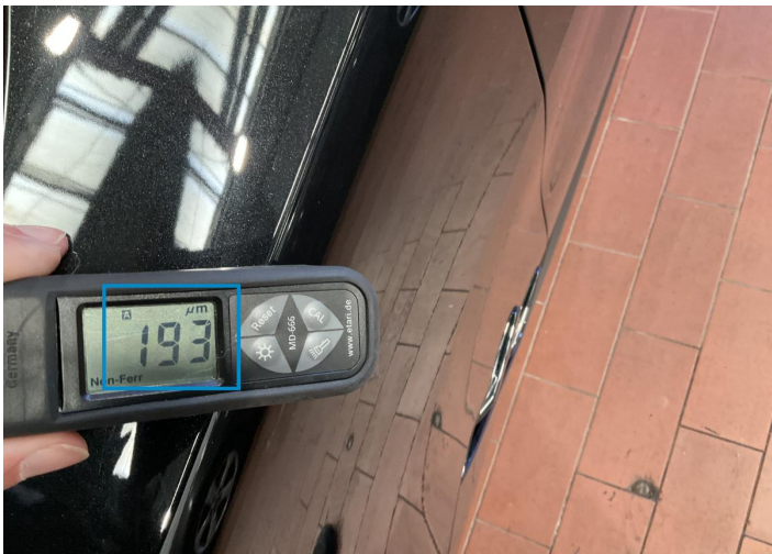
3. Fender / Front Left Paint / Poor Previous Repair -
