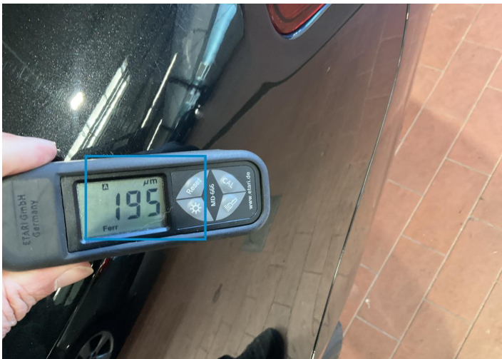
2. Side Panel / Back Left Paint / Poor Previous Repair -
