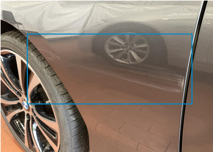
6. Fender / Front Left Paint / Scratch / Scuff -
