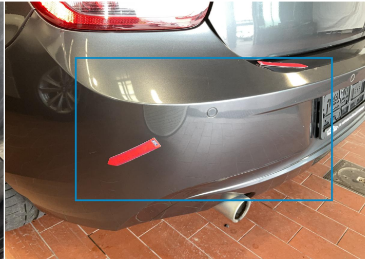
8. Bumper / Back Paint / Scratch / Line -
