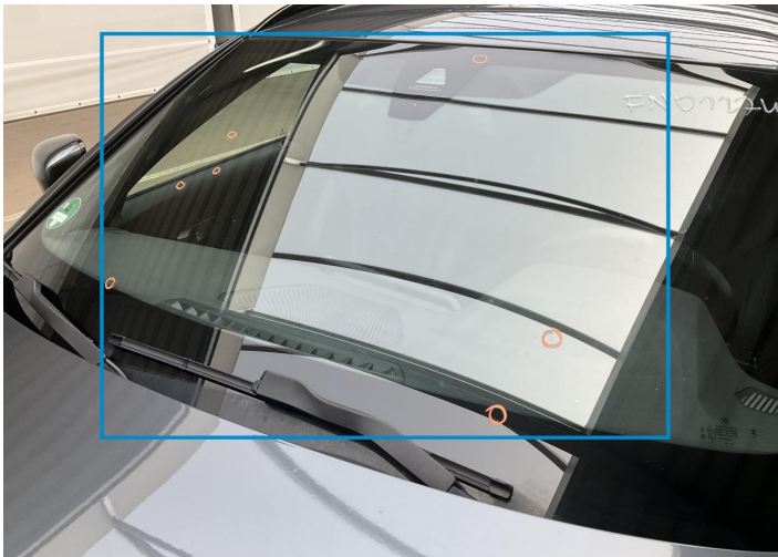
5. Windshield / Front Glass Break / Impact -
