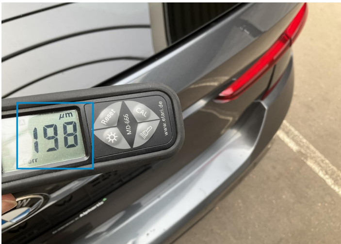
7. Tailgate Paint / Poor Previous Repair -
