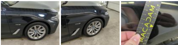
Door FR, Scratch(es), Repair and paint (complete)
