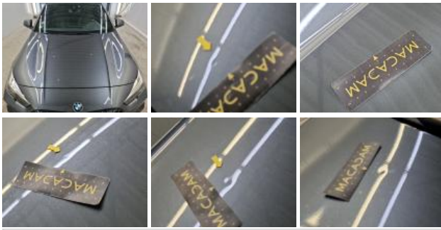
Door FR, Scratch(es), Repair and paint (partial)
