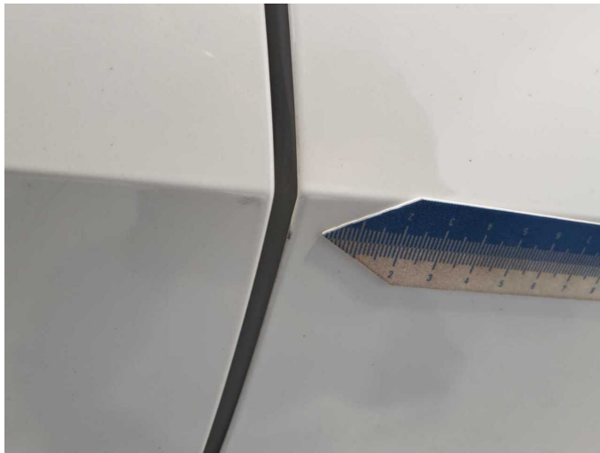
Wear and tear 2: Door - front right side: Door edge - Scratch(es) - No deduction
