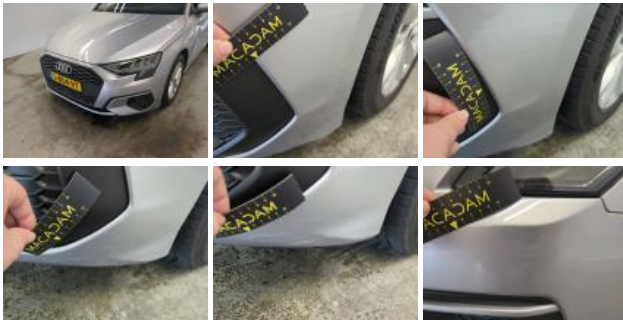
Wing FR, Scratch(es), Repair and paint (complete)
