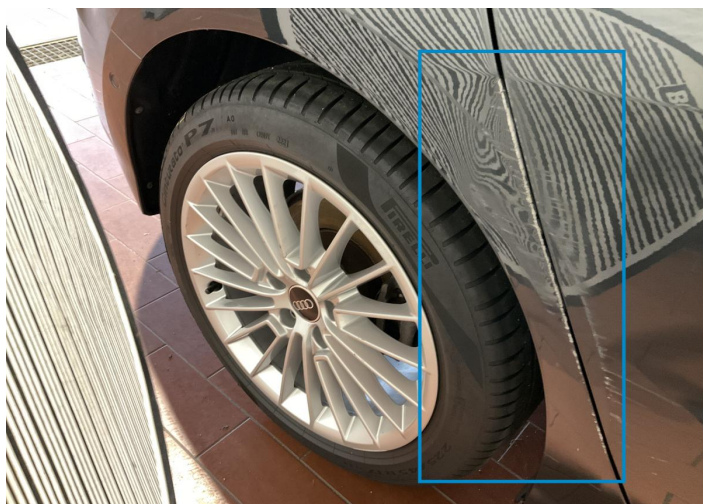
5. Side Panel / Back Right Bodywork / Dent / Dent -
