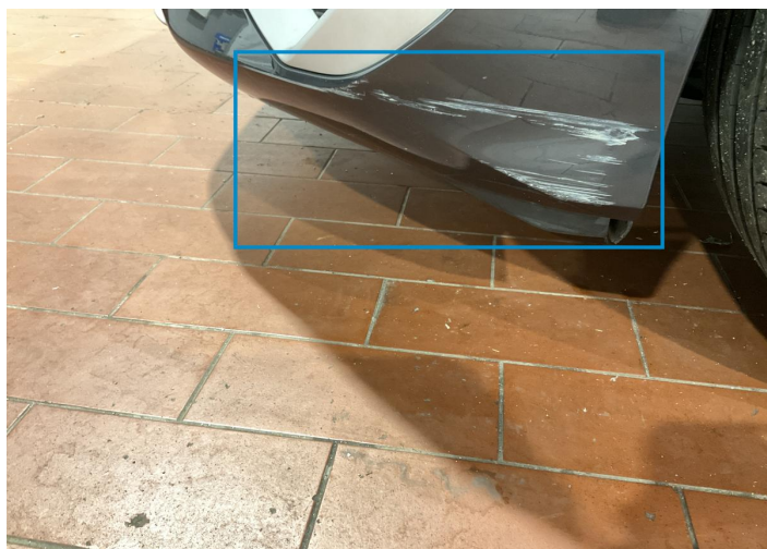
1. Corner Bumper / Front Left Paint / Scratch / Scuff -
