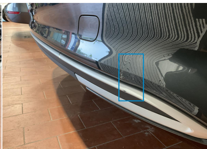
4. Bumper / Back Bodywork / Dent / Dent -
