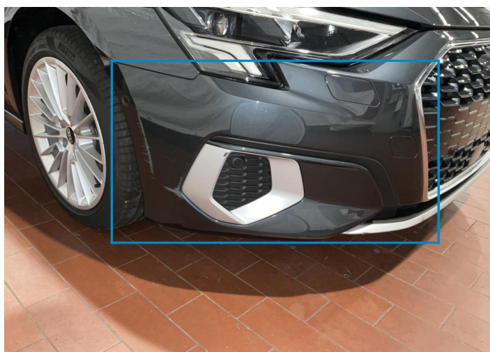
3. Bumper / Front Bodywork / Dent / Dent -
