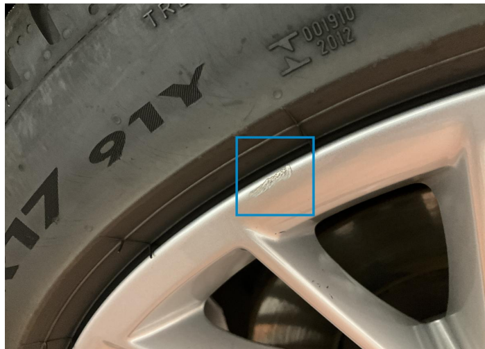
7. Rim / Front Right Paint / Stone Chip -
