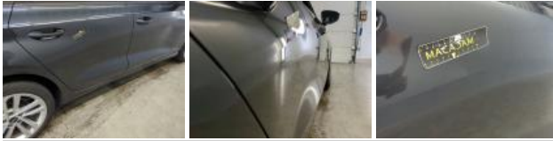
Door FR, Dent(s), Repair and paint (complete)
