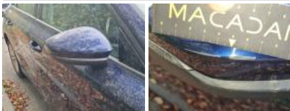
Outside rear-view mirror housing R, Scratch(es), Repair and paint (complete)
