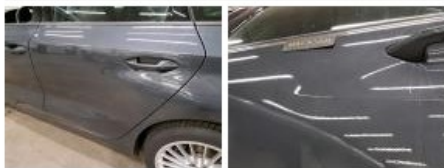
Wing RL, Bad repair, Repair and paint (complete)
