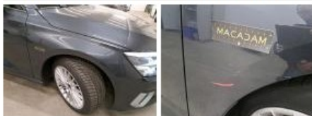
Door FR, Scratch(es), Repair and paint (complete)
