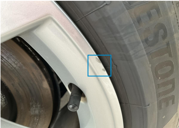
4. Rim / Back Left Out of Bodywork / Scratch -
