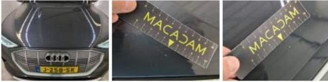
Bumper moulding F, Scratch(es), Replace and paint
