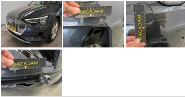
Spoiler FL, Broken, Replace and paint
