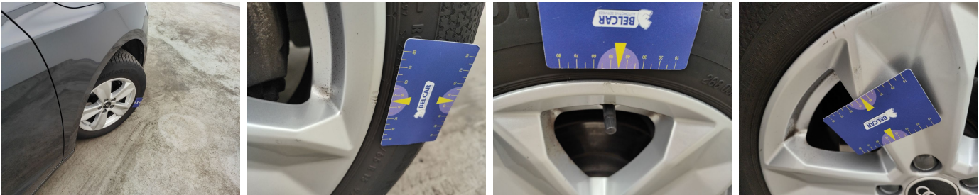
Wheel Alloy Front Right // Repair-scratch
