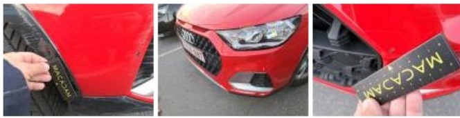
Bumper spoiler F, Scratch(es), Spot repair
