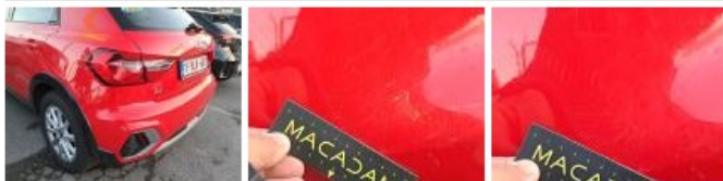
Wing trim FR, Scratch(es), Repair and paint (complete)
