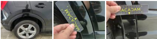
Door trim RR, Scratch(es), Replace and paint
