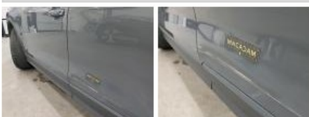
Door FL, Scratch(es), Repair and paint (complete)
