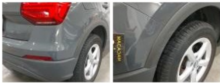
Bumper moulding R, Dent(s) and scratch(es), Replace
