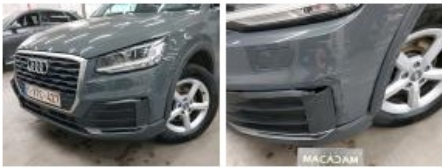
Bumper moulding F, Broken, Replace
