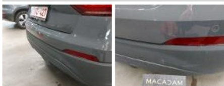
Reflector, Broken, Replace
