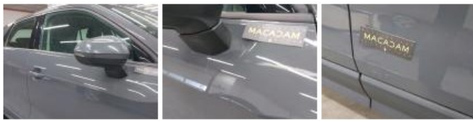
Door RR, Scratch(es), Repair and paint (complete)
