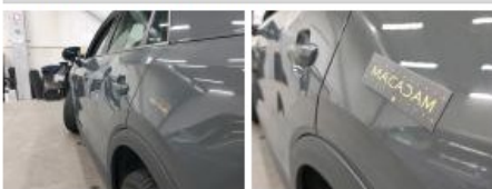
Door RL, Dent(s) and scratch(es), Repair and paint (complete)
