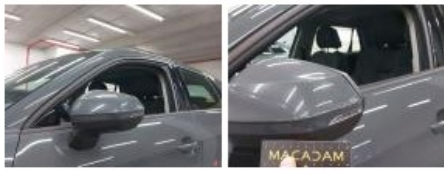
Outside rear-view mirror base L, Scratch(es), Smart repair
