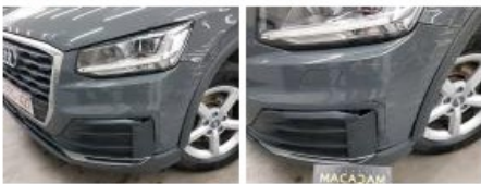
Bumper moulding F, Broken, Replace
