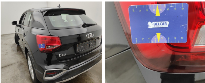
Light / Rear left / Replace-scratch
