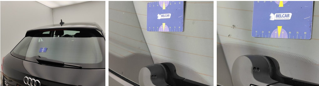
Rear Bonnet / Rear Window / Replace-scratch
