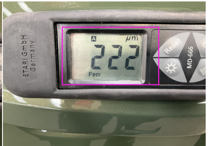
2. Door / Front Left Paint / Poor Previous Repair -
