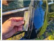
Mirror side repeater R, Broken, Replace
