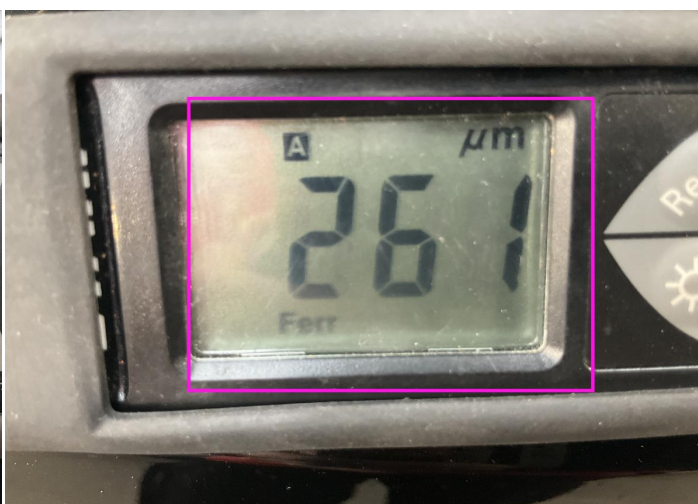
2. Door / Back Left Paint / Poor Previous Repair -
