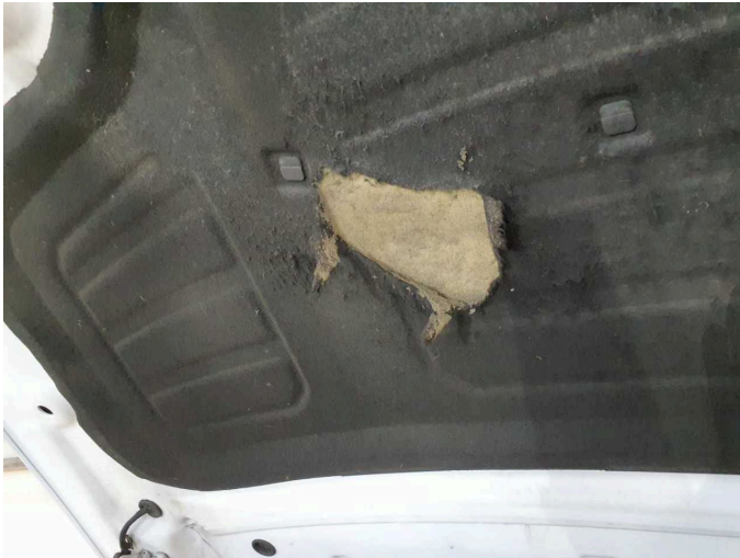
Damage 3: Bonnet: Insulation lining - Broken / torn - Replace
