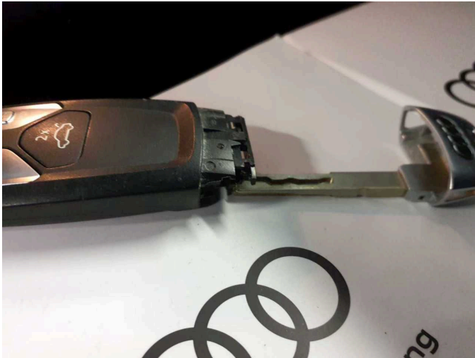
Damage 5: Equipment: Vehicle key - Broken / torn - Replace
