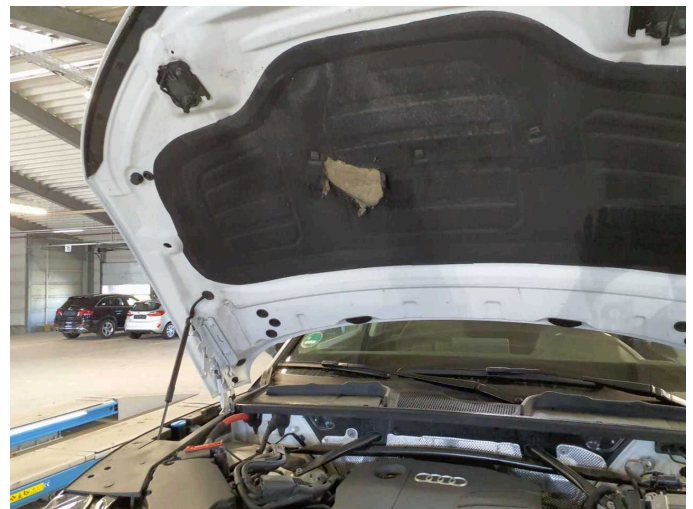
Damage 3: Bonnet: Insulation lining - Broken / torn - Replace
