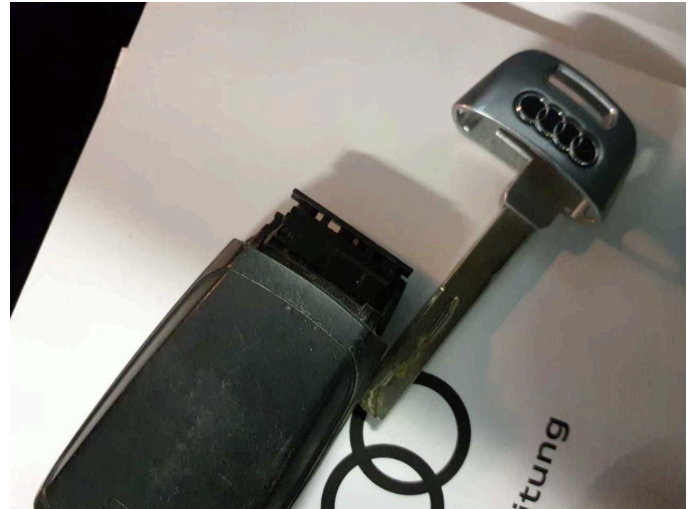
Damage 5: Equipment: Vehicle key - Broken / torn - Replace
