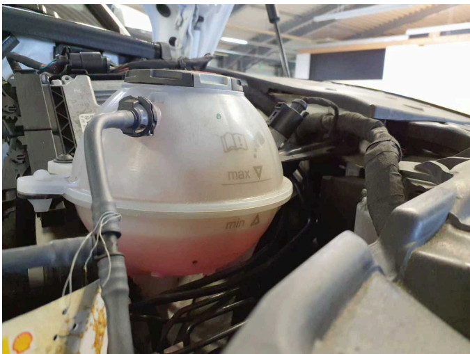
Damage 2: Engine cooling: Coolant - Missing - Perform diagnosis
