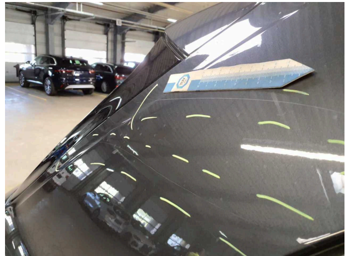
Damage 4: Side panel - rear right side: Side panel (Kratzer) - Dent / paintcoat damage - Repair and paint
