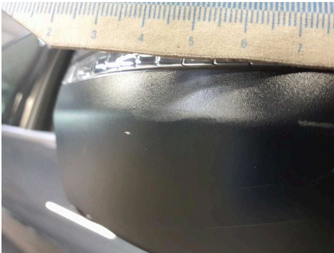
Damage 3: Wing mirror - right side: Mirror housing - Scratched - Replace
