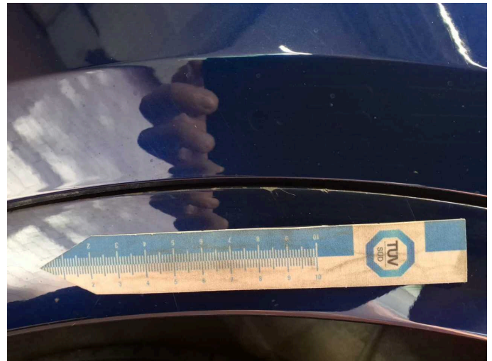
Damage 6: Side panel - rear left side: Wheel well extension - Scratch(es) - Smart repair
