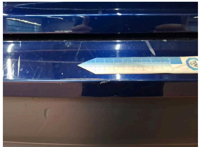
Damage 10: Rear bumper: Rear bumper - Scratched - Paint
