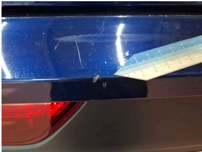
Damage 10: Rear bumper: Rear bumper - Scratched - Paint
