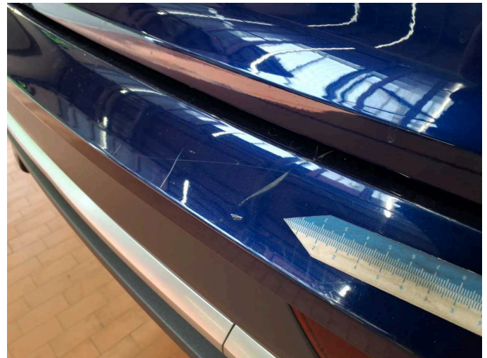
Damage 10: Rear bumper: Rear bumper - Scratched - Paint
