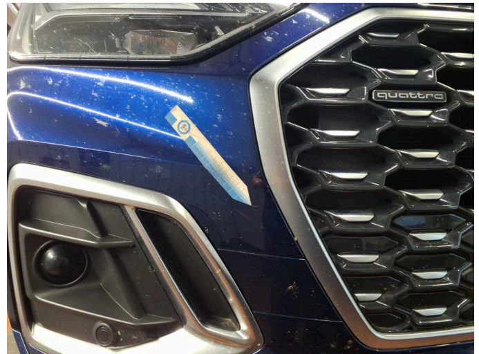
Damage 12: Front bumper: Front bumper - Scratched - Paint
