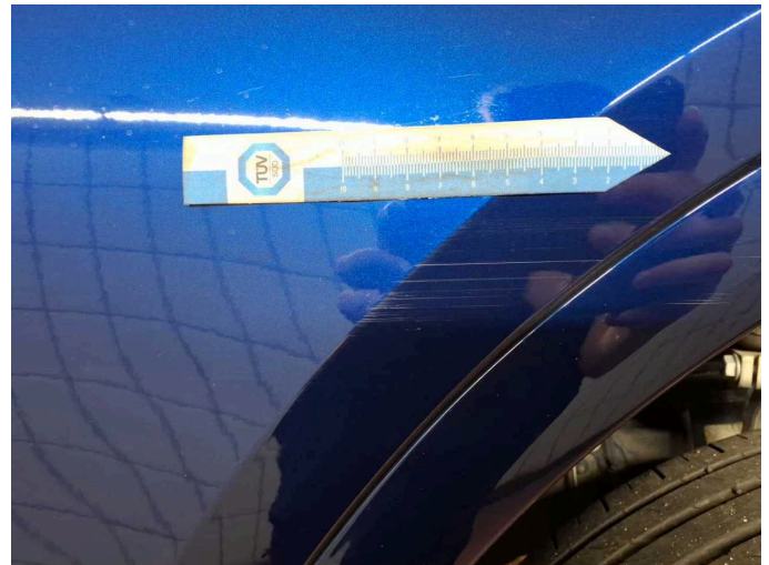
Damage 13: Mudguard - right side: Mudguard - right side - Scratched - Paint
