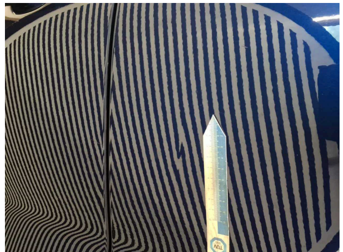
Wear and tear 5: Door - rear left side: Door - dent(s) - Smooth repair work
