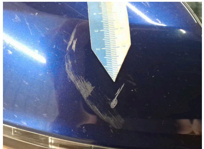
Damage 2: Wing mirror - right side: Cap - Scratch(es) - Paint
