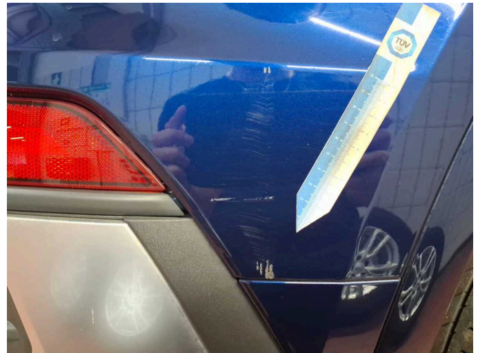
Damage 10: Rear bumper: Rear bumper - Scratched - Paint
