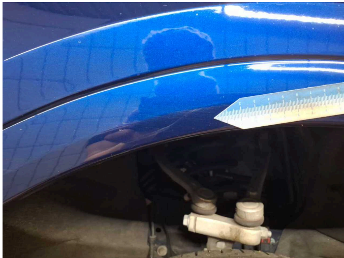
Damage 3: Mudguard - right side: Wheel well extension - Scratched - Smart repair
