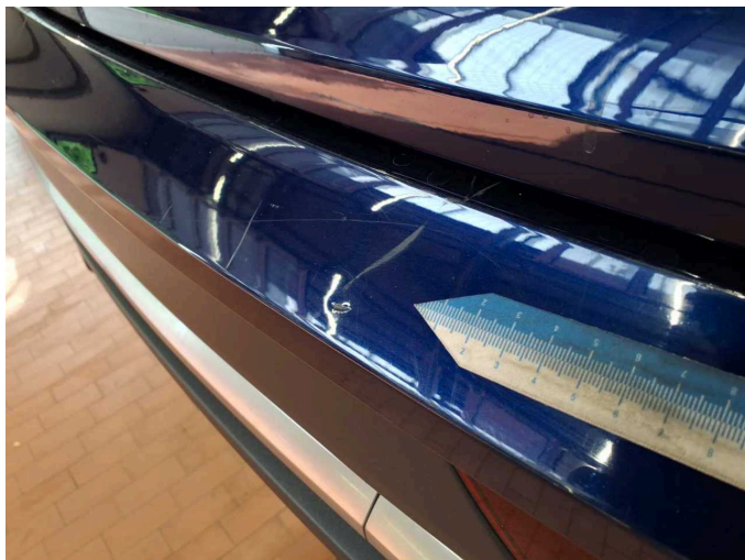
Damage 10: Rear bumper: Rear bumper - Scratched - Paint
