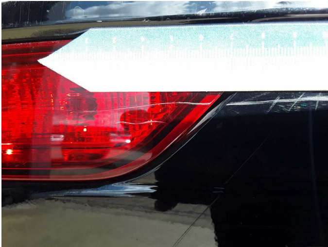
Damage 4: Rear bumper: Reflector - left side - Scratch(es) - Replace
