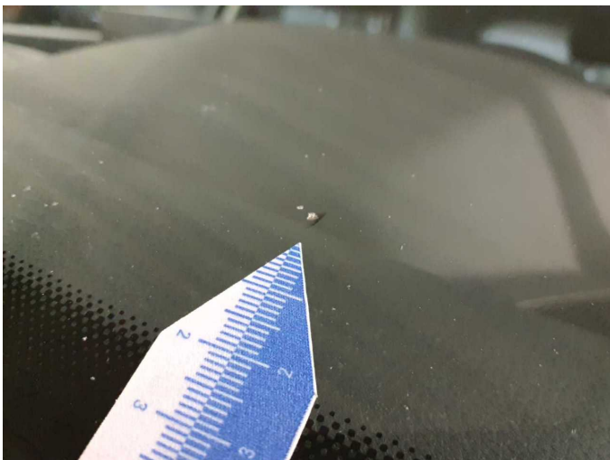
Damage 8: Vehicle glazing: Windscreen - Stone chips - Replace
