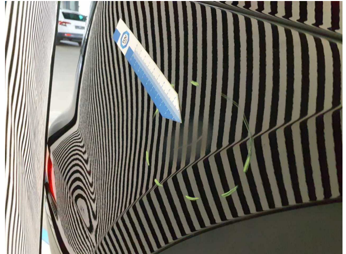
Damage 6: Rear bumper: Rear bumper - Scratched - Paint
