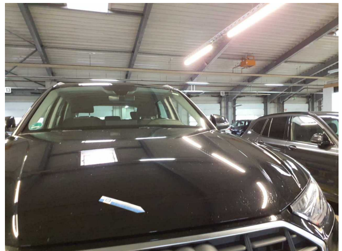
Damage 7: Bonnet: Bonnet (Steinschlag) - Scratched - Paint
