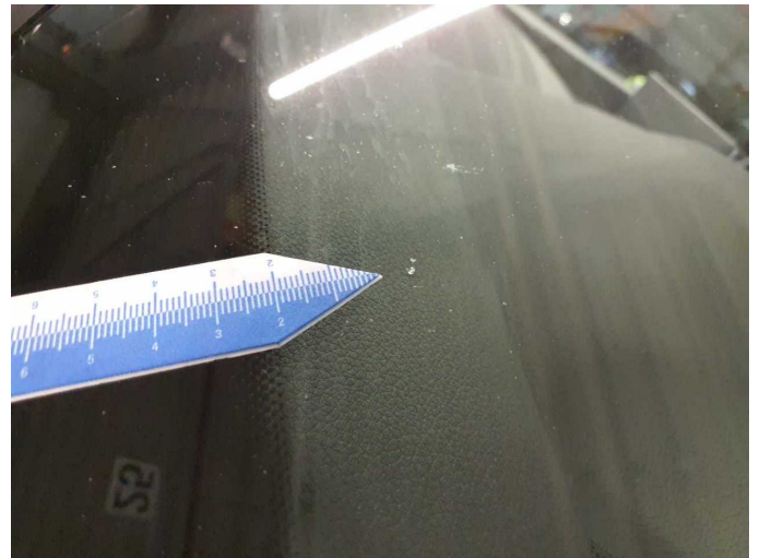
Damage 8: Vehicle glazing: Windscreen - Stone chips - Replace
