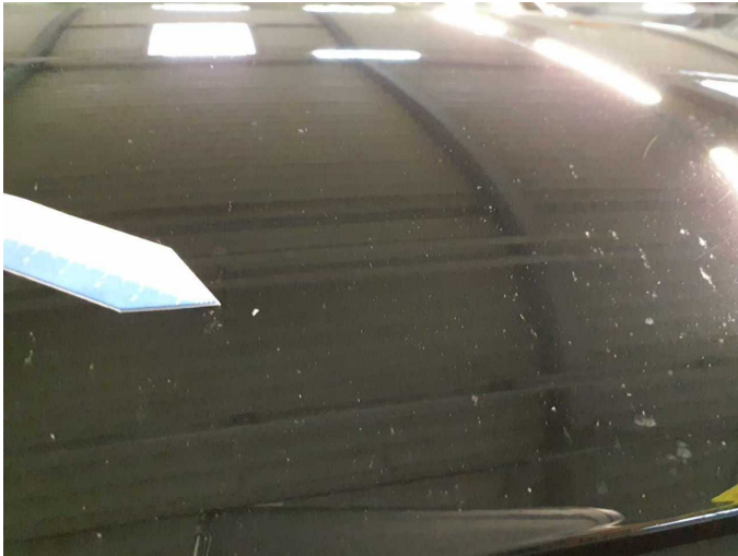
Damage 7: Bonnet: Bonnet (Steinschlag) - Scratched - Paint
