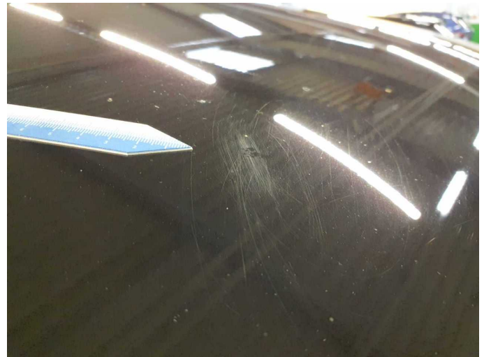
Damage 7: Bonnet: Bonnet (Steinschlag) - Scratched - Paint
