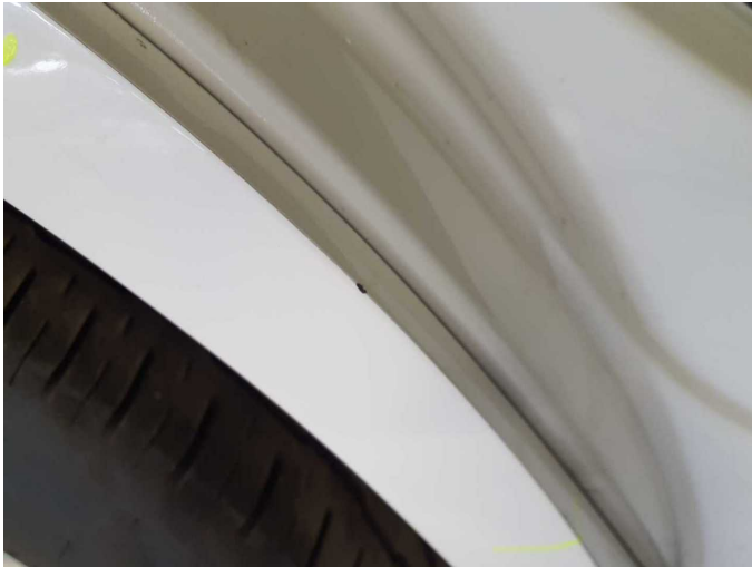
Damage 3: Side panel - rear right side: Wheel arch - Scratch(es) - Smart repair
