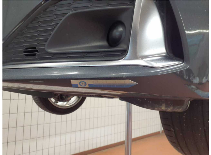
Damage 14: Front bumper: Front bumper - Scratched - Paint
