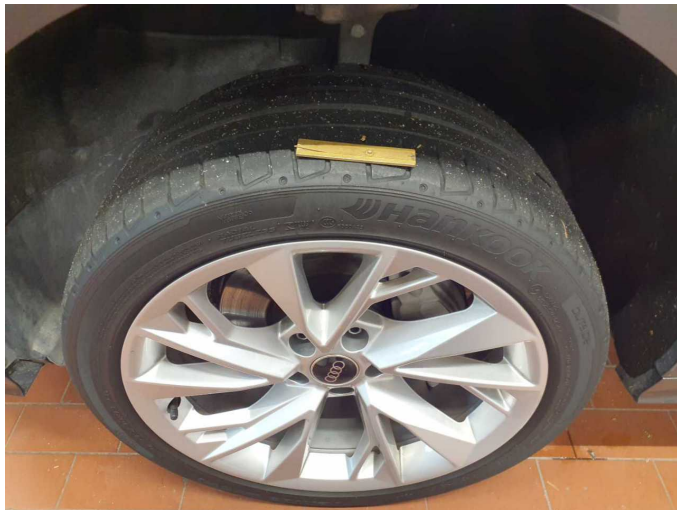
Damage 3: Wheel / tyres: Tyre - front left side (2mm) - Does not meet the leasing specifications - Replace
