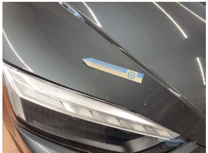
Damage 15: Bonnet: Bonnet - Stone chips - Paint
