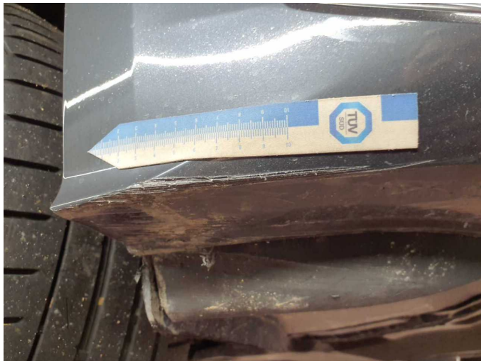
Damage 14: Front bumper: Front bumper - Scratched - Paint
