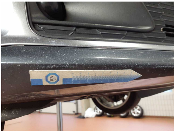
Damage 14: Front bumper: Front bumper - Scratched - Paint
