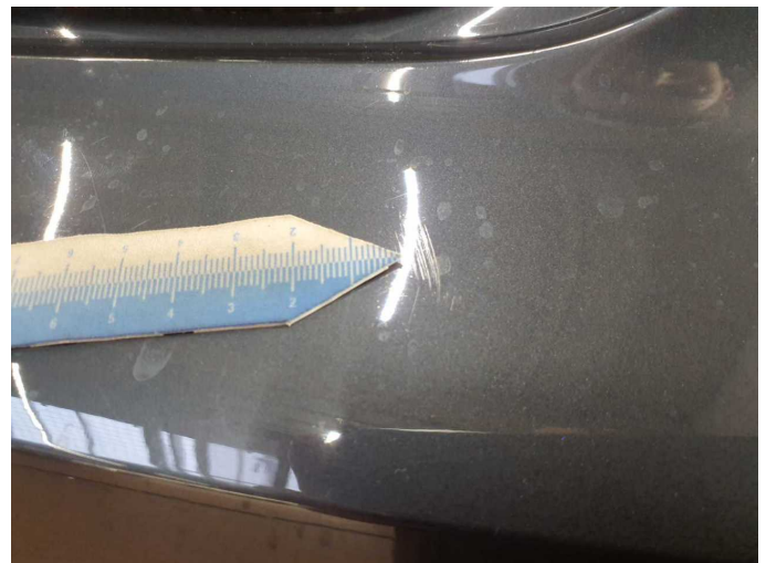
Damage 13: Rear bumper: Rear bumper - Scratch(es) - Paint
