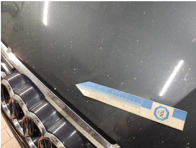
Damage 15: Bonnet: Bonnet - Stone chips - Paint
