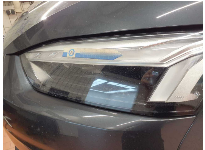
Damage 5: Headlight: Headlight - left side - Stone chips - Loss in value
