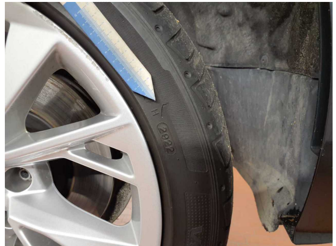
Damage 2: Wheel / tyres: Tyre - front right side - Broken / torn - Replace
