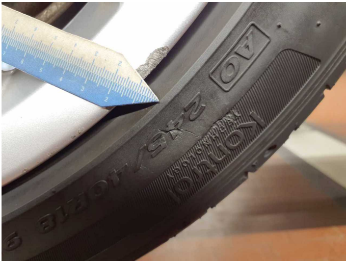
Damage 1: Wheel / tyres: Tyre - rear right side - Broken / torn - Replace
