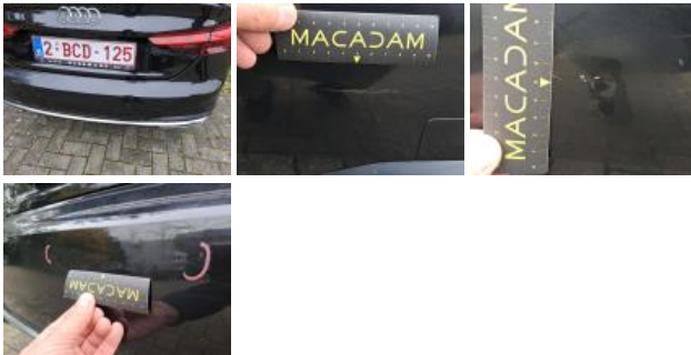
Wheel aperture RR, Scratch(es), Spot repair
