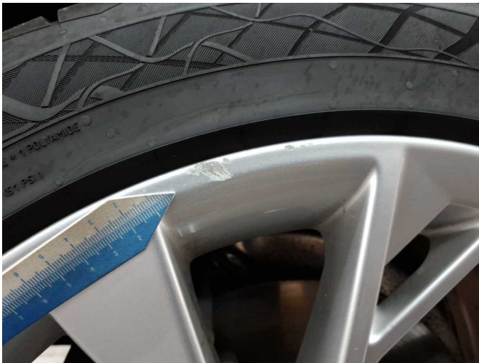
Wear and tear 2: Wheel / tyres: Alloy rim - front right side - Scratch(es) - No deduction
