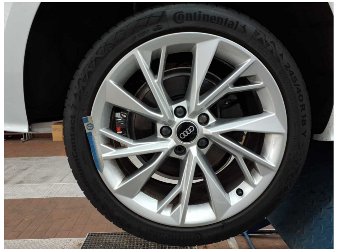
Wear and tear 3: Wheel / tyres: Alloy rim - rear right side - Scratch(es) - No deduction
