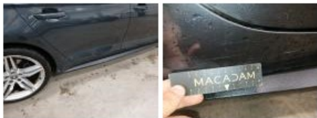
Alloy rim FR, Scratch(es), Repair and paint (complete)
