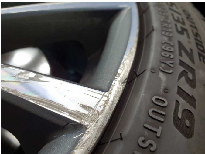
Damage 7: Wheel / tyres: Alloy rim - front right side (Materialabtrag) - Damaged - Replace
