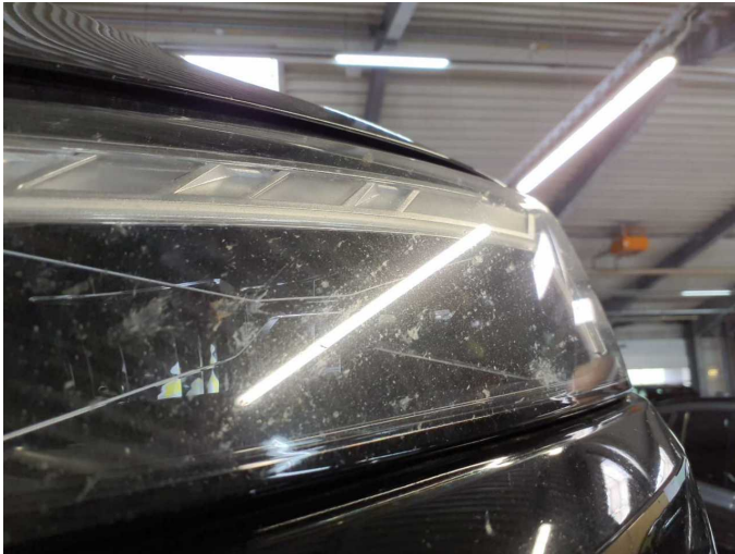
Wear and tear 4: Headlight: Headlight - left side - Stone chips - No deduction
