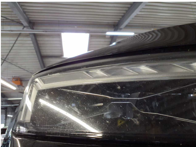
Wear and tear 3: Headlight: Headlight - right side - Stone chips - No deduction
