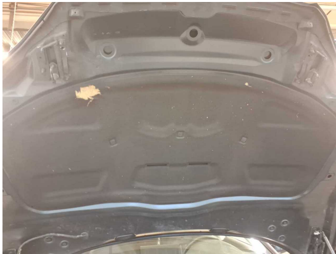
Damage 8: Bonnet: Insulation lining - Damage caused by marten / rodent - Replace
