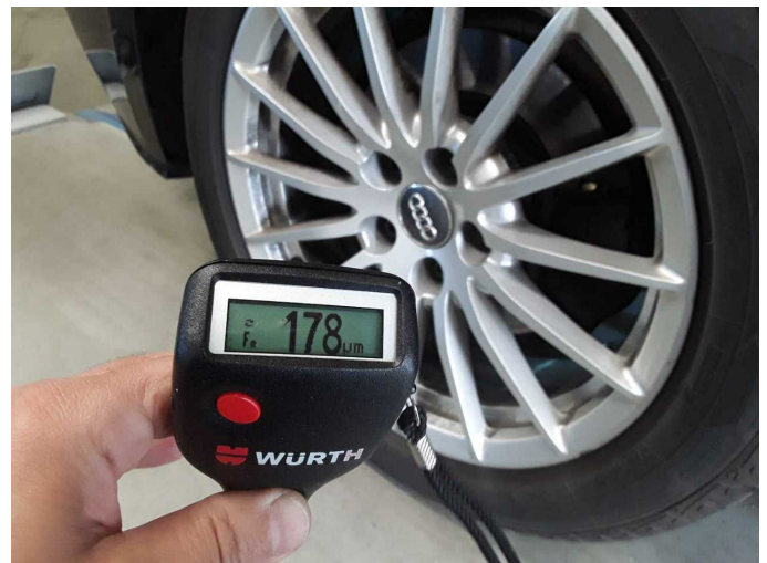
Side panel - rear right side: 178 µm
