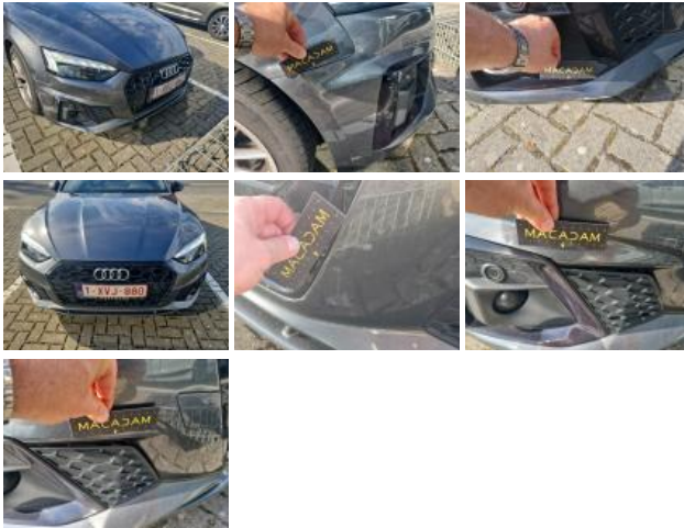
Bumper moulding F, Scratch(es), Replace
