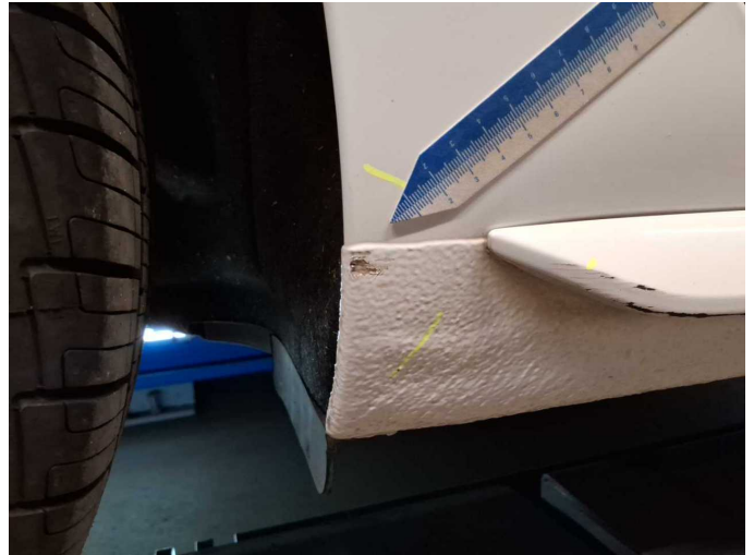
Damage 9: Sill - right side: Sill (und Leiste) - Dent / paintcoat damage - repair according to calculation
