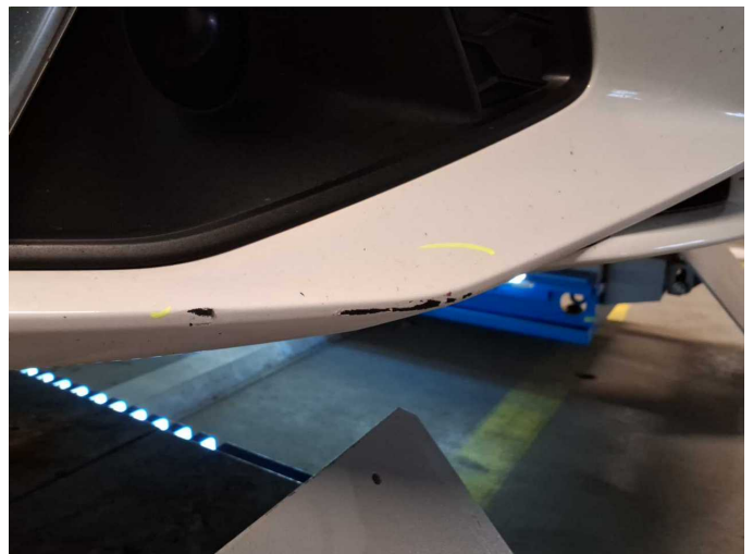
Damage 10: Front bumper: Front bumper - Scratched - Paint
