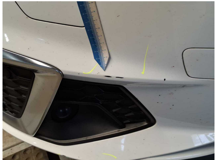
Damage 10: Front bumper: Front bumper - Scratched - Paint
