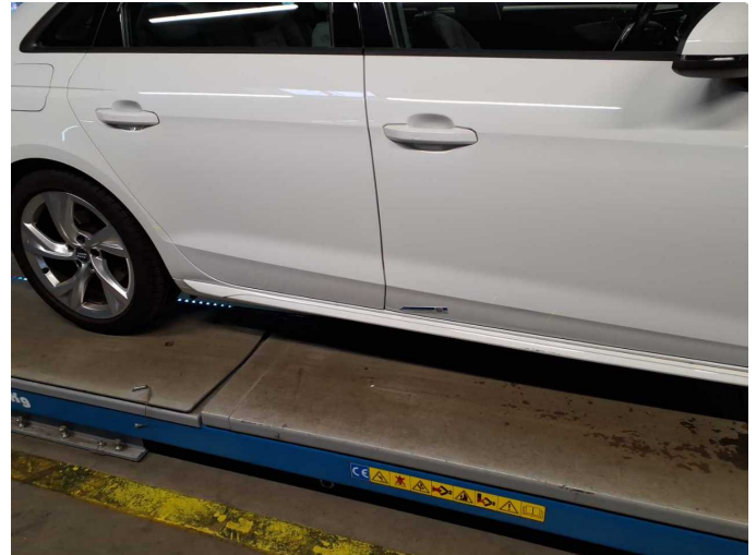
Damage 7: Door - front right side: Door - Deformed - Repair and paint
