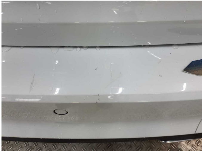
Damage 5: Rear bumper: Rear bumper - Scratch(es) - Paint
