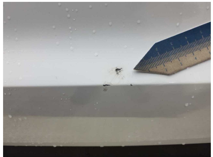
Damage 5: Rear bumper: Rear bumper - Scratch(es) - Paint
