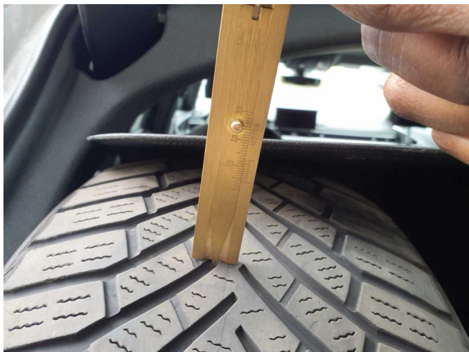
Wear and tear 2: 2nd wheel set: 2 tyres (Nicht Bestandteil der Ausstattung) - Does not meet the leasing specifications - No deduction
