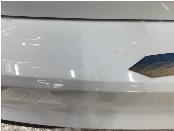
Damage 5: Rear bumper: Rear bumper - Scratch(es) - Paint
