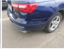
Bumper R, Scratch(es), Repair and paint (complete)
