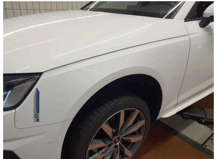
Damage 1: Mudguard - left side: Mudguard - left side - Stone chips - Smart repair
