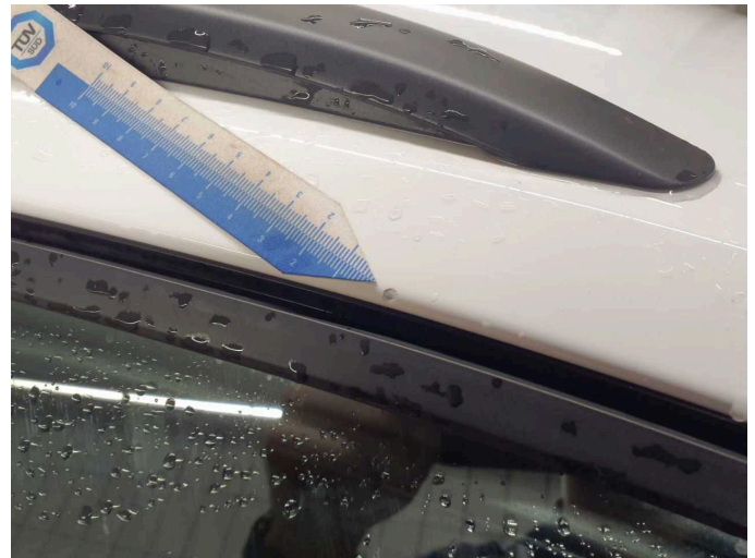
Damage 5: Roof: Roof rail - right side - Dent / paintcoat damage - Repair and paint
