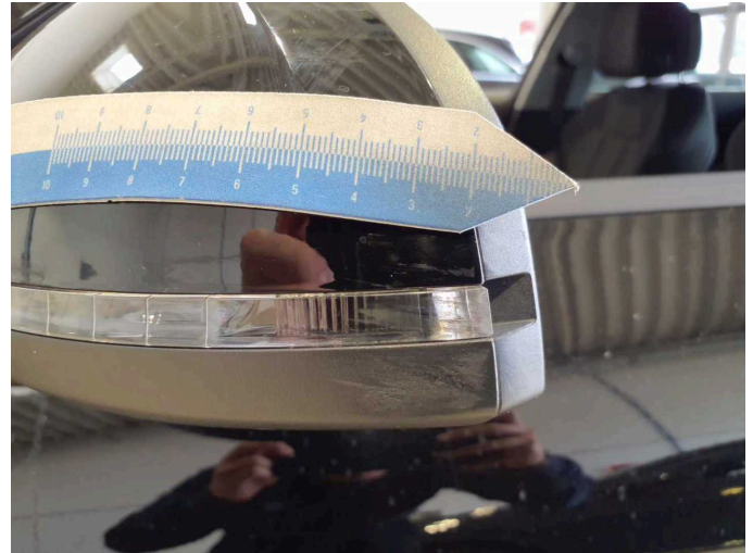
Damage 6: Wing mirror - left side: Wing mirror - Damaged - Replace
