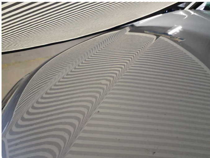
Damage 4: Bonnet: Bonnet - dent(s) - Smooth repair work
