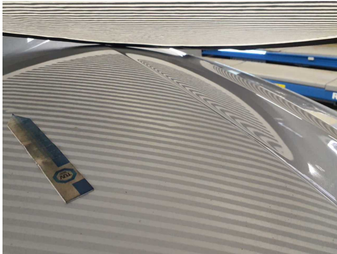
Damage 4: Bonnet: Bonnet - dent(s) - Smooth repair work
