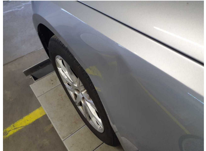
Damage 5: Mudguard - left side: Mudguard - left side - Deformed - Replace
