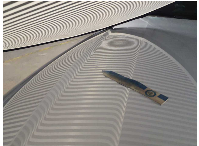
Damage 4: Bonnet: Bonnet - dent(s) - Smooth repair work
