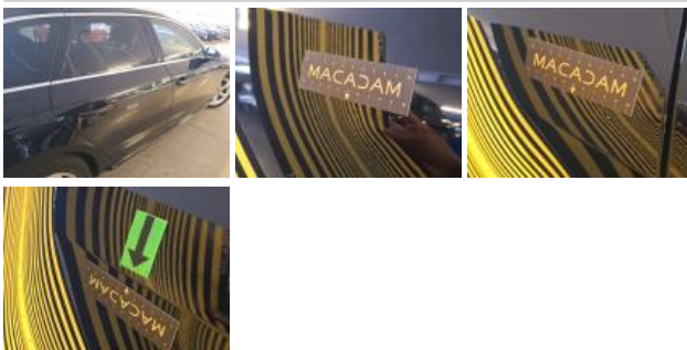
Door RR, Dent(s), Paintless dent repair
