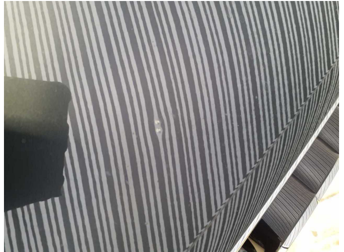
Damage 14: Bonnet: Bonnet (+ Steinschläge) - Dent / paintcoat damage - Repair and paint
