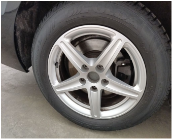
Wheel Rear Right / Hub Cover with Logo / Replace-missing
